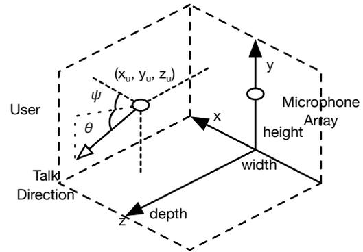
Figure 3: Coordinate system used in data collector:
